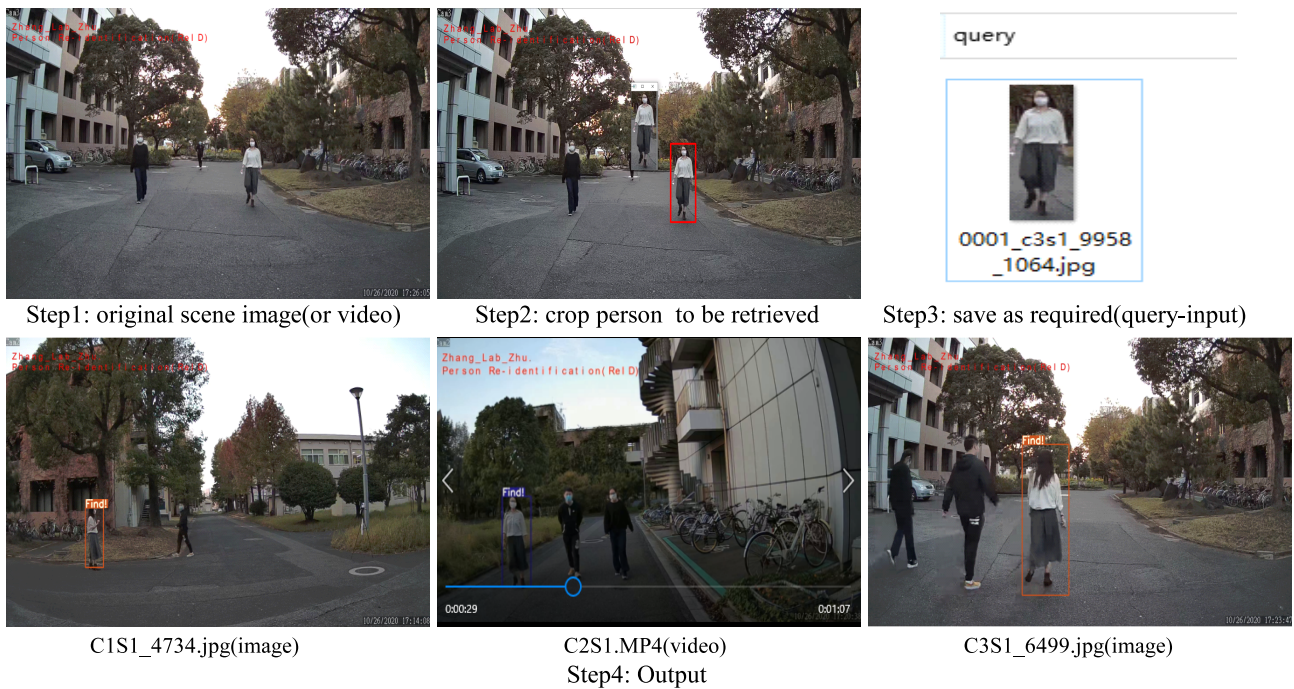
Fig. 6 Experiment in real-world application scenario, the search results come from gallery multiple non-overlapping cameras
