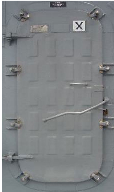
Fig. 7. Picture of a quick-acting watertight door. Originally published by Pier Side Supply in [52].
