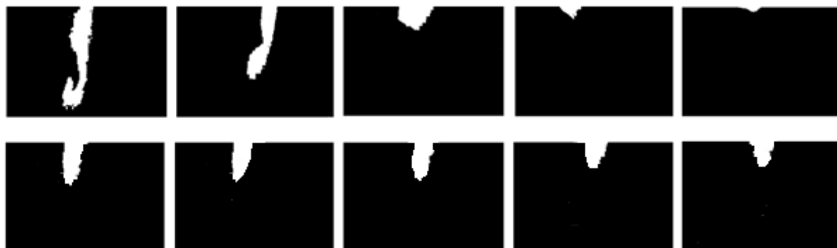
Fig. 42. Images from real dataset at 350W (top) at 0.2, 0.4, 0.6, 0.8, and 1.0 m/s, with images generated by CVAE (bottom) from each class
