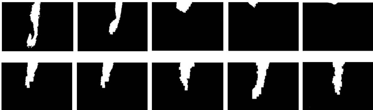
Fig. 41. Images from real dataset at 350W (top) at 0.2, 0.4, 0.6, 0.8, and 1.0 m/s, with images generated by VAE (bottom) from that training data
