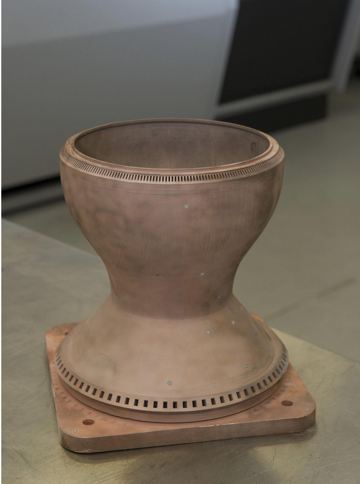
Fig. 2. 3-D printed rocket nozzle made from copper material
