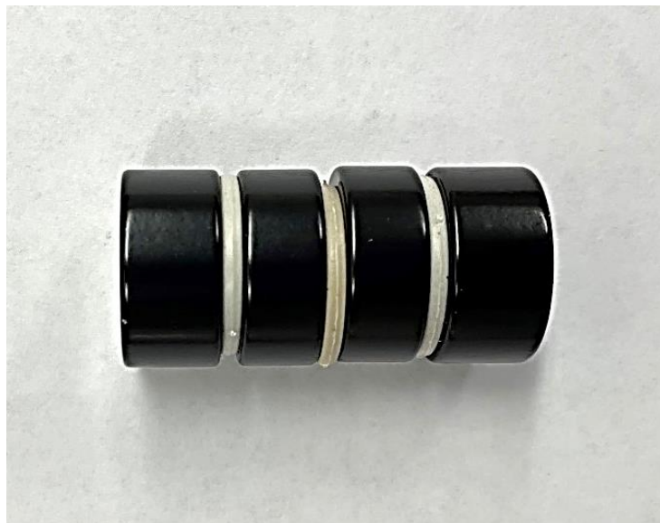
Fig. 6.6. Picture of the magnets used in the magnetron. The white materials are washers used to separate the magnets from each other.
