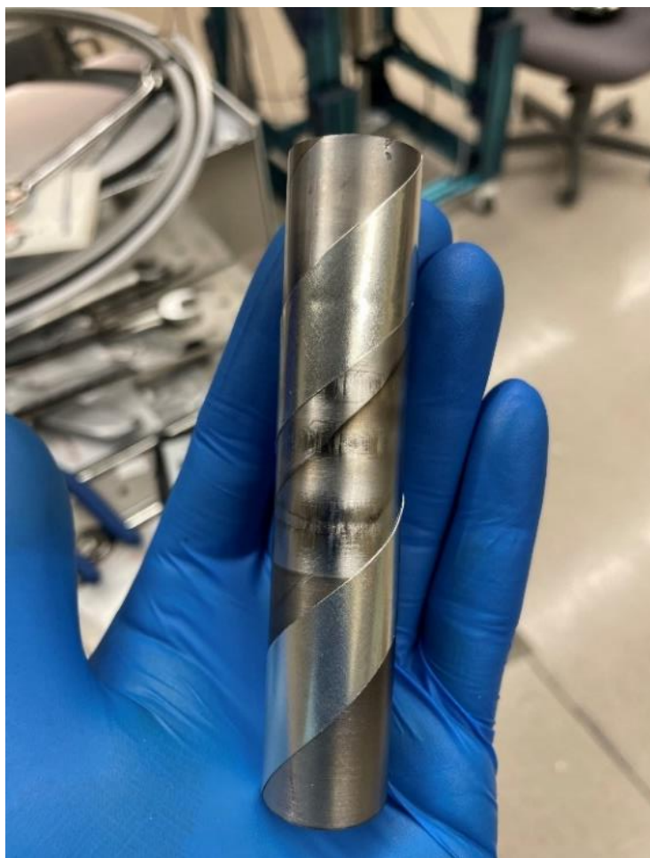
Fig. 6.11. Sn target made of by wrapping Sn foil helically on Nb tube target.
