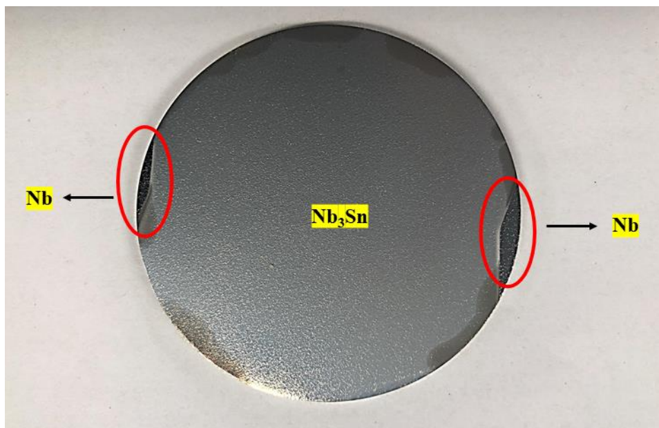
Fig. 7.7. Picture of the Nb 3 Sn film coated for the RF surface impedance measurement. The exposed Nb substrate near the uncoated region is clearly seen from the picture.
