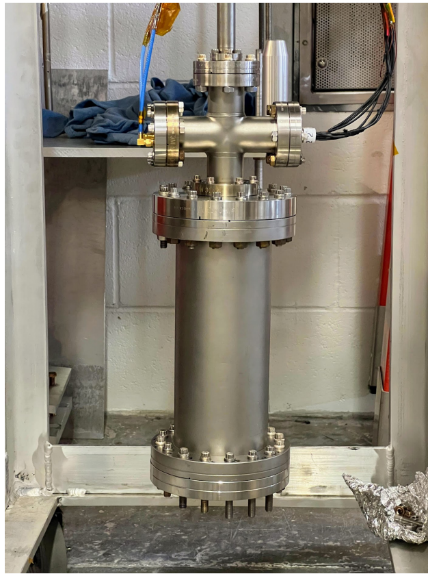
FIG. 32: The vacuum chamber connected to the vertical test stand for testing.
