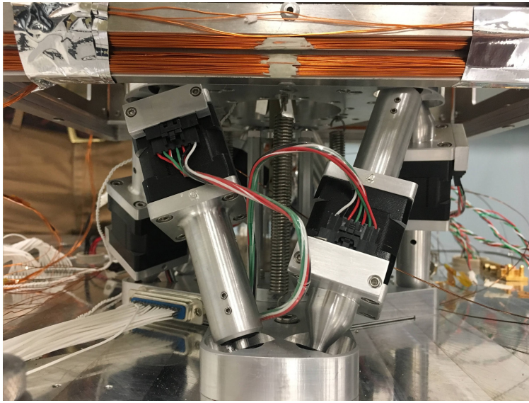
FIG. 59: Mini Hexapod MHP-14, a six-actuator kinematics platform, that is used to fine adjust the angles and the positions of the superconducting magnet during sample measurements.
