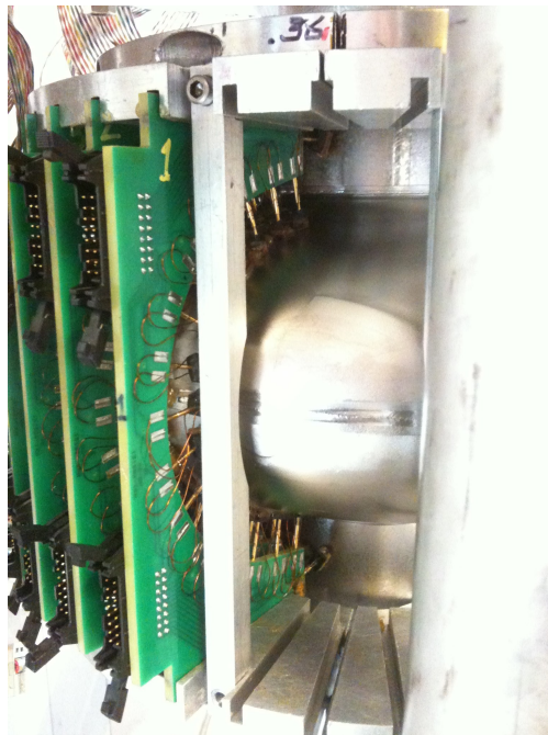
FIG. 14: A single-cell cavity with a partially attached thermometry system.
