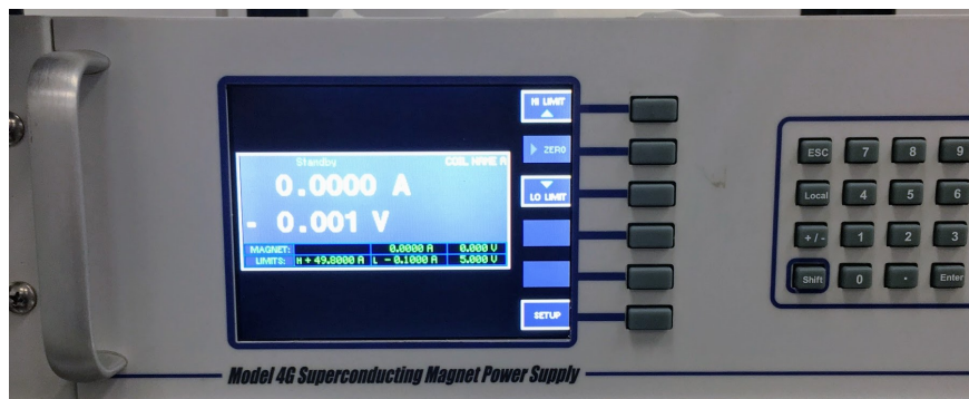
FIG. 57: A magnet power supply for the superconducting magnet which is used to operate the ramp up and down of the magnet.
