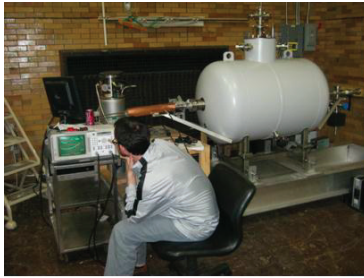
Figure 7: Eigenmode spectrum measurements of the multi-spoke cavity in the full cryomodule assembly at room temperature.
