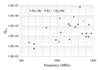
Figure 6: Required Q<sub>ext</sub> for HOMs to achieve the specified damping.
