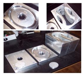
Figure 4: 800 MHz elliptical shaped cavity prototype.
