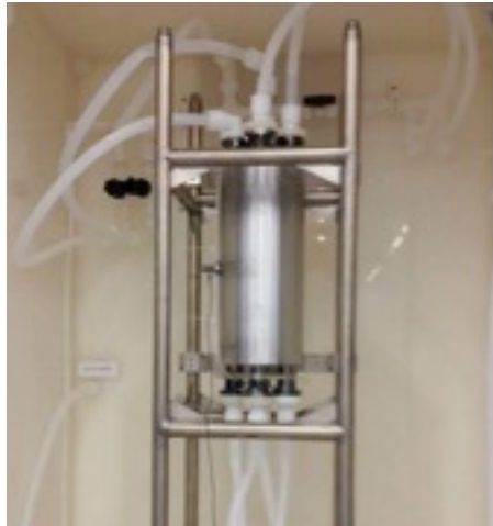
Figure 2: BCP set up in the clean room.
