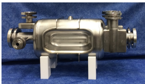
Figure 1: 400 MHz prototype rf-dipole cavity.
