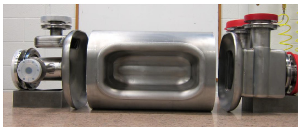
Figure 3: Sub-assemblies of the rf-dipole cavity.
