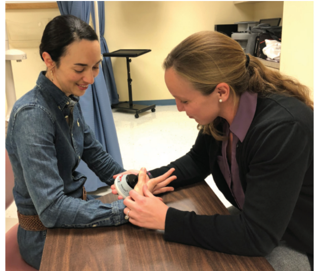
Figure 5: Handheld dynamometer for measuring muscle force production
