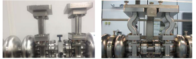
FIG. 3. Close-up picture of the FPC waveguide section for original C20 cavities (left) and after the refurbishment using doglegs (right) as installed in C50 and C75 cryomodules.
