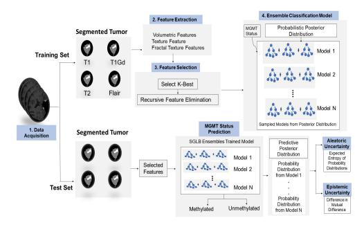
Figure 1: The overall pipeline for MGMT status prediction.
