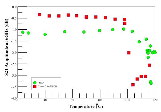
**Figure 1.** Temperature dependence of microwave insertion loss (S21 amplitude) of ZnO on Si substrate in nitrogen-rich air and gaseous ethanol environments, monitored at 6 GHz. Note that the symbol sizes are much larger than the error bars.
