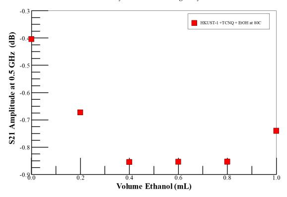
**Figure 3.** Insertion loss (S21 amplitude) monitored at 0.5 GHz as a function of volume of neat ethanol injected into vapor reactor (i.e., ethanol vapor concentration) environments at  $80 \, \text{C}^{\circ}$  in air.
