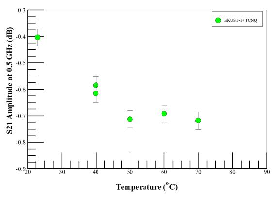
**Figure 2.** Temperature dependence of microwave insertion loss (S21 amplitude) in TCNQ-loaded HKUST-1 MOF on a Si sample in  $N_2$ -rich air. The error bars represent the standard deviation of three or more measurements on the same sample.
