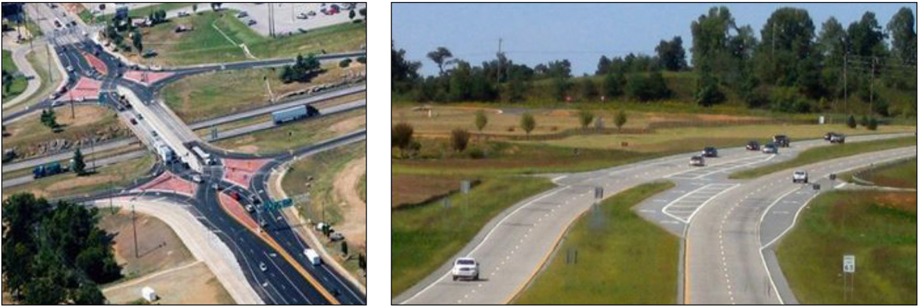
Figure 3: Examples of Intersection Geometry Measures (left to right): Diverging Diamond Interchange (Adapted from Anderson et al., (2012) Offset Left Turn Lanes (Adapted from Creative Commons CC-BY-SA-2.5)
