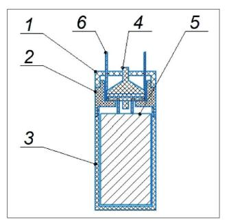
Fig. 2. Hybrid supercondenser on the basis of nanosize nickel hydroxide: 1 - cap; 2 - holder of valve; 3 - glass; 4 - a valve for discharge of excessive pressure;
