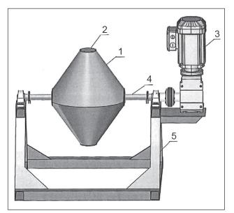
Fig. 1. A device for obtaining nanodispersed powders, with working bicone tool: 1 - welded shell of stainless steel in the shape of bicone; 2 - loading system; 3 - engine; 4 - shaft; 5 - foundation slab
