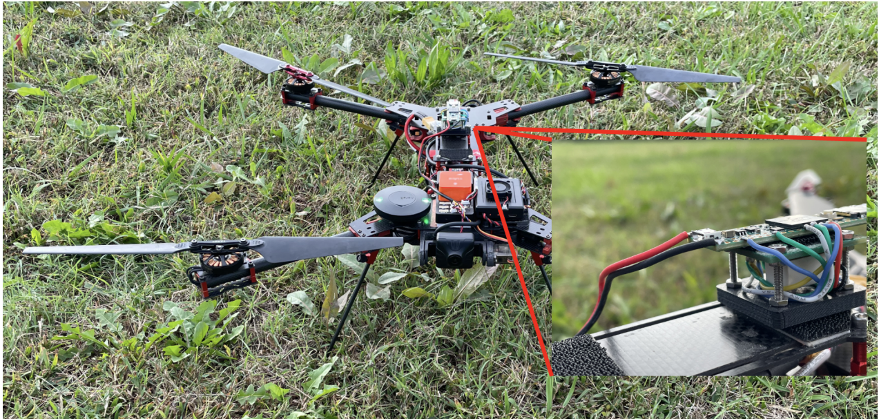
Fig. 15: Additional Quadcopter with Teesny IMU Interface Blown Up
