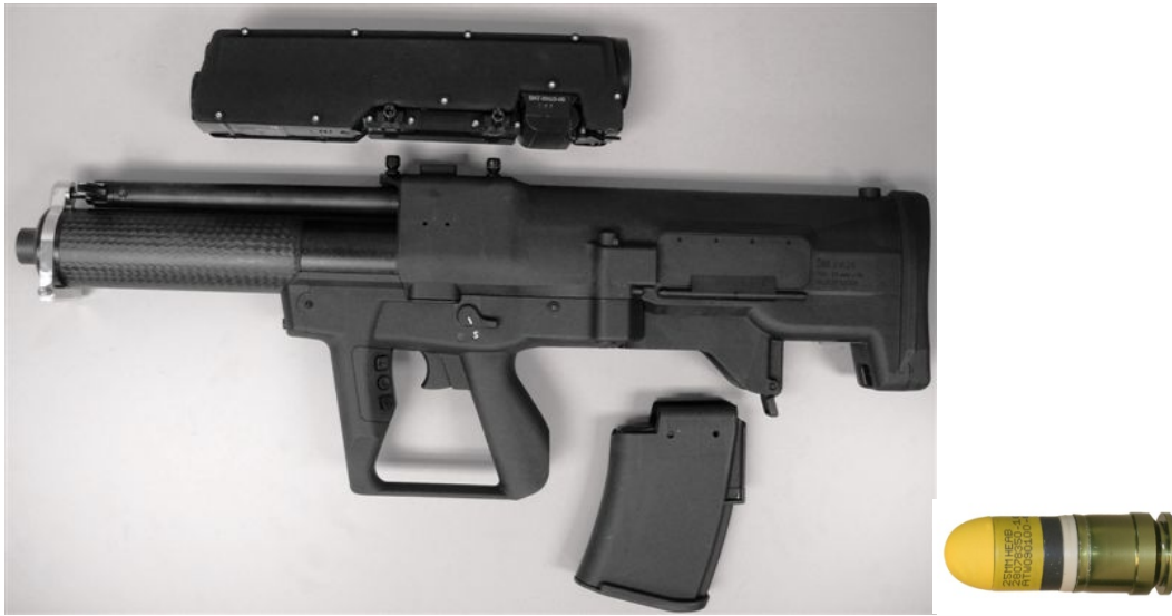
Fig. 2. XM-25 Weapon system and 25mm HEAB Round
