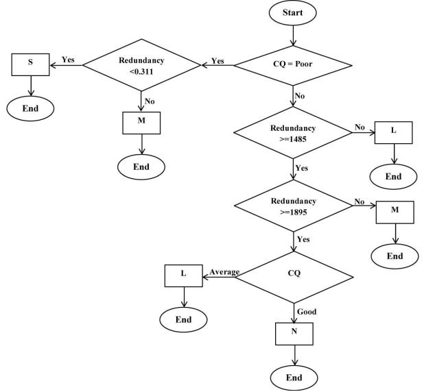
Fig. 6. The proposed flowchart to specify the class of damage state.
