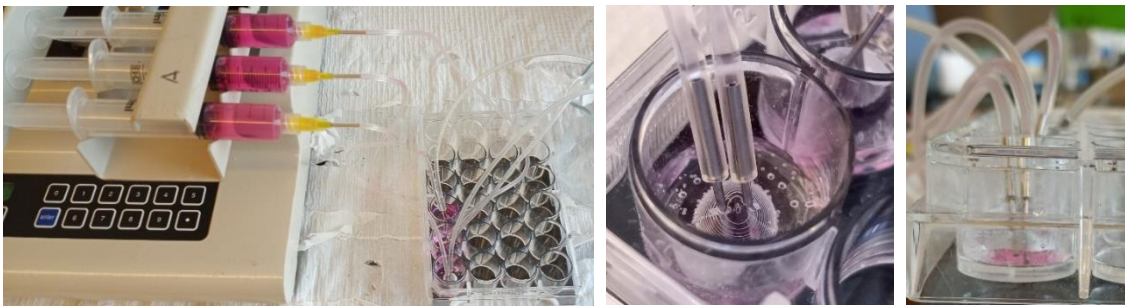
Figure 3.3. The dynamic cell culture design. Close up image of the cell culture chambers in each well. Cells are cultured on the bottom of the plate. Constant fluid flow was maintained within the chamber and throughout the tubing. The total volume within each well was 400 \mu\text{L} .
