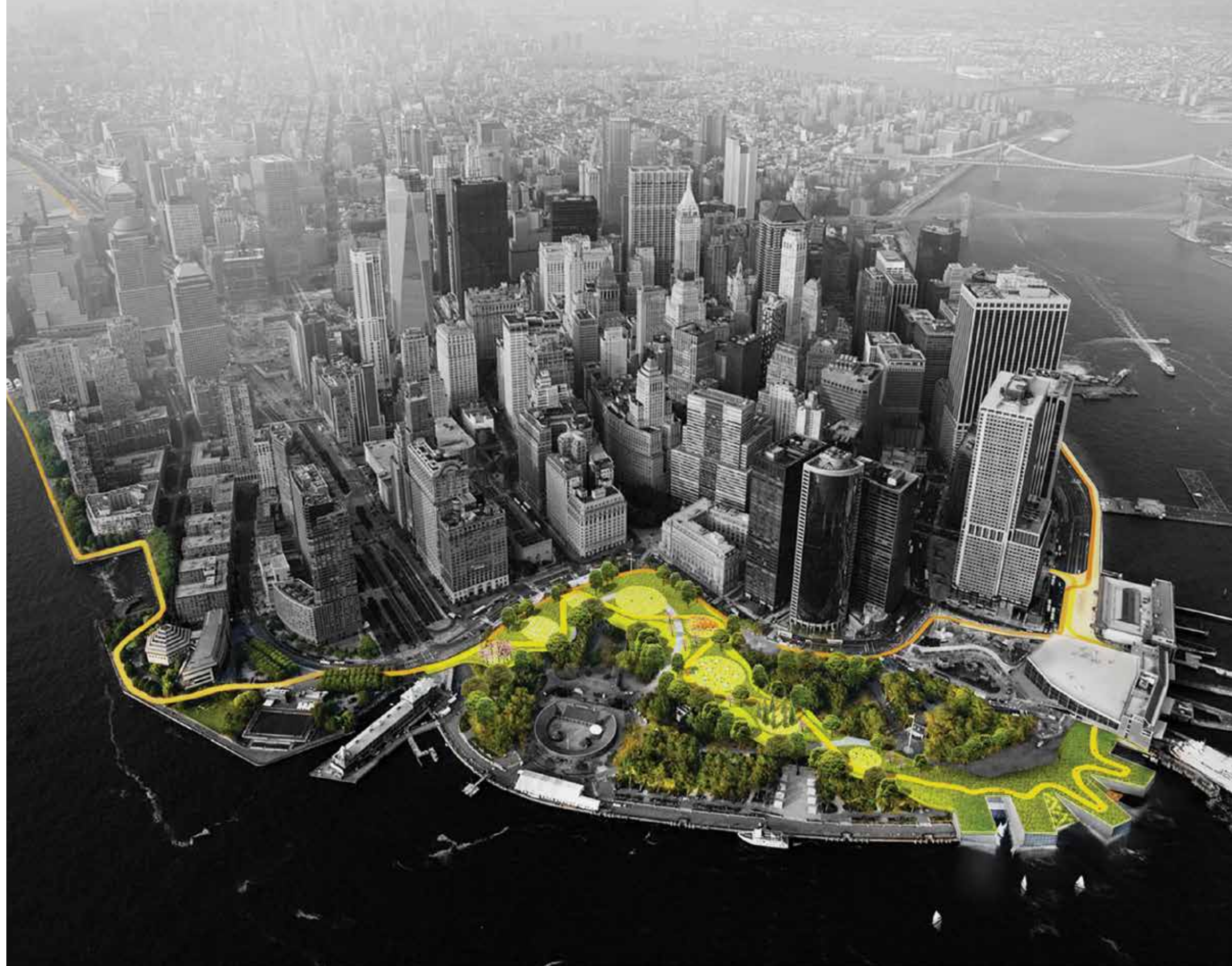
The Big U is one of the winning projects of Rebuild by Design. It combines a continuous 10-mile long flood protection infrastructure along Lower Manhattan with new open spaces and public programs to benefit surrounding communities
