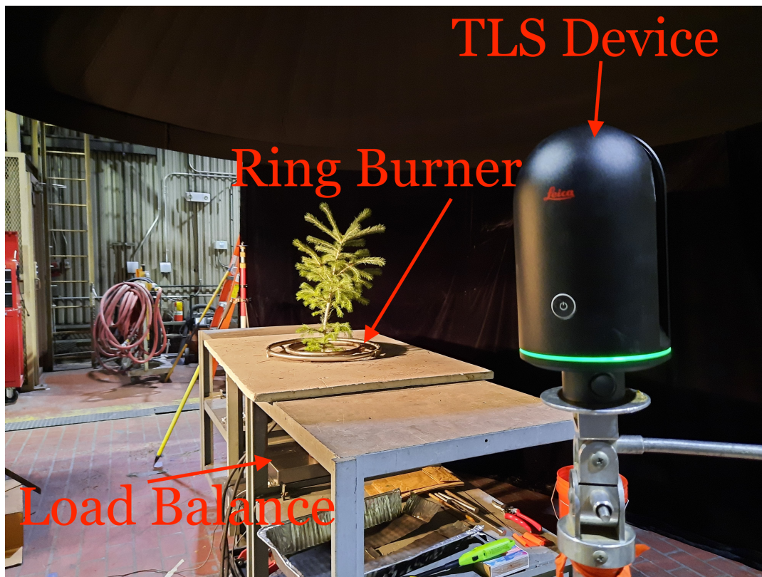
FIGURE 2.3: Photograph of the experimental design at the Missoula Fire Sciences Laboratory.
