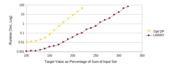
Figure 3.5: A plot of the run times of unbounded subset sum algorithms, the y-axis showing log-scaled run time in seconds and the x-axis showing increasing size of target value as a percentage of the input set sum. The input set was static, comprising  $\{2x10^6 : x \in \mathbb{Z}, 30 \le x \le 48\}$ . Target values were  $\{10x10^7 : x \in \mathbb{Z}, 40 \le x \le 300\}$ , each one guaranteed to return at least one combination.
