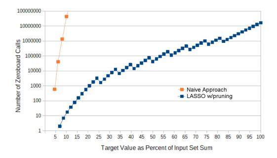
Figure 3.7: A plot of the log-scaled number of Zeroboard hash-table calls by target value as a percentage of the input set sum. Note the comparison between the number of calls made by the naive approach and the pruning approach that LASSO performs. The input values were the set  $\{2x10^6 : x \in \mathbb{Z}, 5 \le x \le 24\}$ , and the target values were  $\{2x10^7 : x \in \mathbb{Z}, 1 \le x \le 29\}$ .
