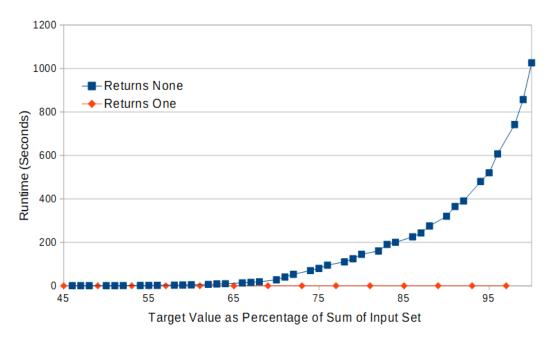
Figure 3.8: A plot of the normalized run time of the modified algorithm that returns only a single valid subset if it exists, showing normalized run time measured over target values generated for every percentile of the input set sum. The input values were the set  $\{2x10 : x \in \mathbb{Z}, 1 \le x \le 19\}$ , and the target values started at 200, incrementing by 55 up to the sum of the input set.
