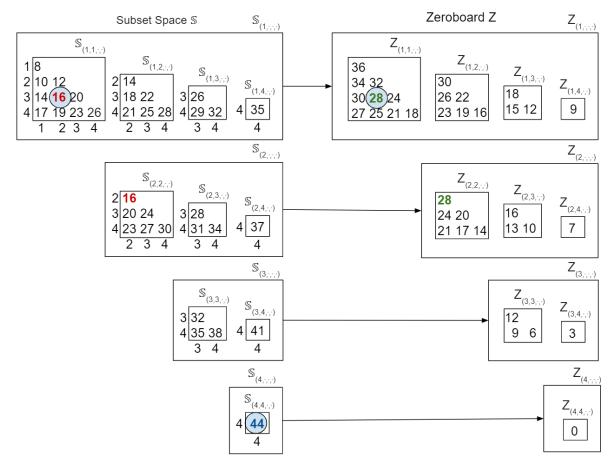
Figure 2.1: An example of the subset space S and an equivalent Zeroboard, both containing subsets of size four. Note the definitions of nomenclature that describe individual subsets and groups of subsets found in the subset space S and the Zeroboard space Z.
