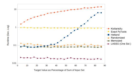
Figure 3.2: A plot of the run times of bounded subset sum algorithms showing log-scaled run time in seconds by increasing size of target value as a percentage of the input set sum. The inputs set remained static over all targets. All target values are guaranteed to return at least one subset.
