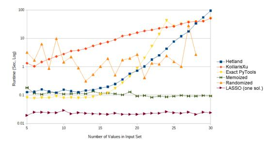
Figure 3.1: A plot of the run times showing the log-scaled run time of bounded subset sum algorithms in seconds by increasing size of the input set. Note that LASSO is modified to return a single result. The input sets used comprised  $\{2x10^6 : x \in \mathbb{Z}, 5 \le x \le 4+n\}$  where n ranged from 5 to 30 as seen on the x-axis. The target value was calculated as the sum of the inputs, divided by 2 and rounded up to the nearest subset sum guaranteed to return at least one combination.
