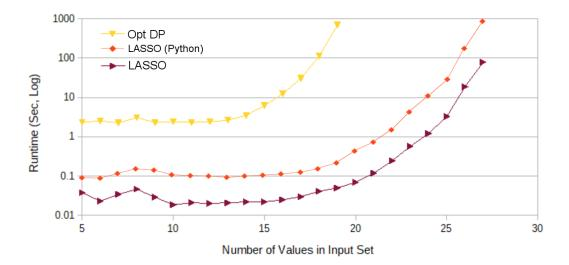
Figure 3.4: The run time of unbounded subset sum algorithms in seconds by increasing size of the input set. The input sets used comprised  $\{2x10^6 : x \in \mathbb{Z}, 5 \le x \le 4+n\}$  where n ranged from 5 to 30 as seen on the x-axis. The target value was calculated as the sum of the inputs, divided by 2 and rounded up to the nearest subset sum guaranteed to return at least one combination.
