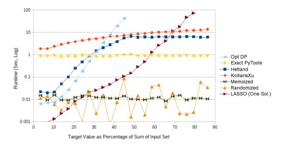
Figure 3.10: A plot of the run times of all competing algorithms showing the log-scaled run time in seconds by increasing size of target value as percentage of input set sum. The input set was static, comprising  $\{2x10^6 : x \in \mathbb{Z}, 5 \le x \le 24\}$ . Target values were  $\{(2x10^7)+1 : x \in \mathbb{Z}, 2 \le x \le 50\}$ , each one guaranteed to return no combination.
