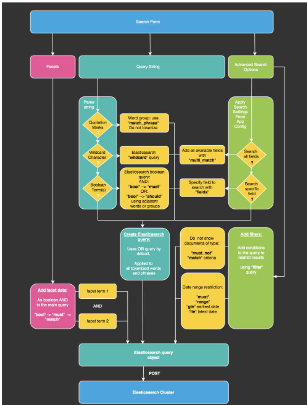
Figure 5. Flow to construct an Elasticsearch query object. The code checks the query string, also if any facets or advanced search parameters exist and their conditions. The query object is sent to the Elasticsearch cluster to get back a JSON response of search results.
