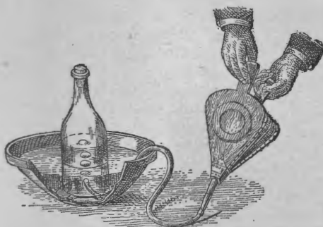
3. Collecting and measuring gas.
