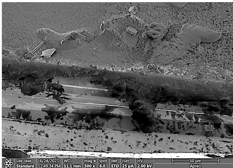
Figure 18. Profile views using SEM. Conditions of drying: 70 degrees Celsius, on silicon wafer.
