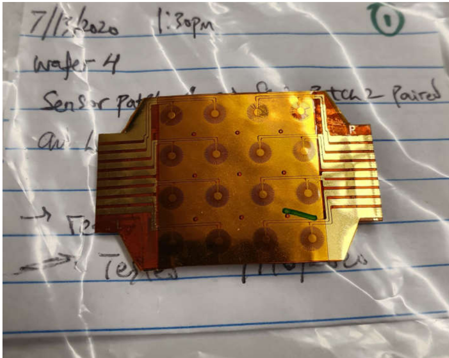
Figure 2: NGS-produced SkinCell, 4 by 4 skin sensors with 3.5mm vertical and horizontal spacing between each sensor
