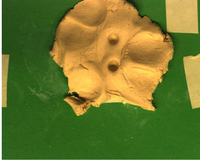
Figure 48: Clay indentions to extract pixel per millimeter ratio
