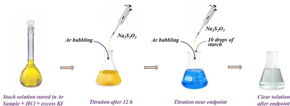
Figure 2.3.4: Schematics showing the steps in iodometric titration.
