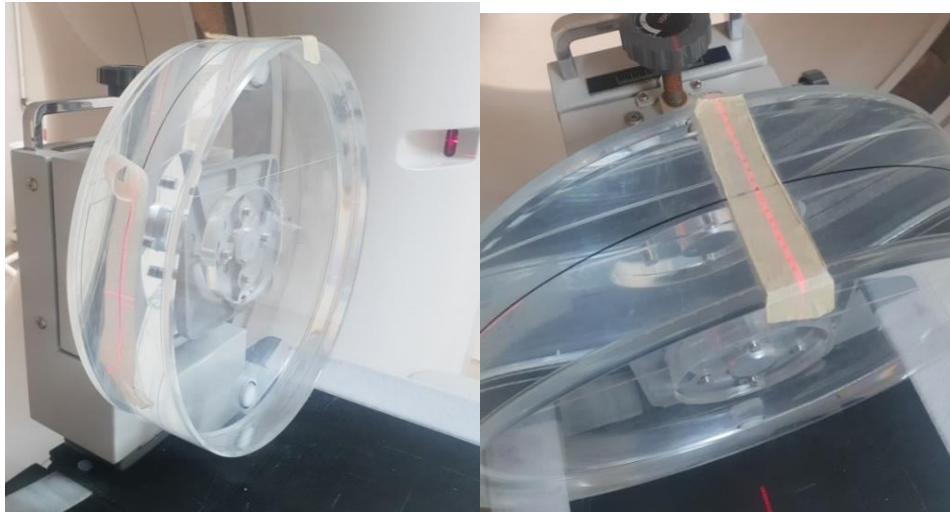
Figure 2.5: Water phantom set-up with red laser, lateral and anterior view. (Courtesy of the researcher, photos taken during research).
