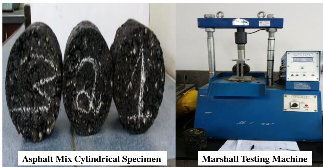
Figure 5. 1. Asphalt Cylindrical Specimen Mounted on the Marshall Stability and Flow Testing Machine (Source: Author, 2019)
