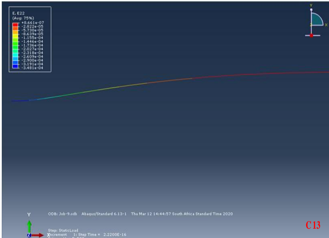
Appendix C12 – C13. Vertical Compressive Strain at the Top of 150 mm WMA – 30% RAP Pavement Structure
