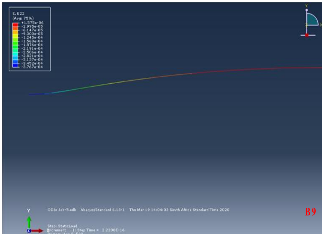
Appendix B8 – B9. Vertical Compressive Strain at the Top of Sub- Grade of 100 mm WMA – 15% RAP Pavement Structure
