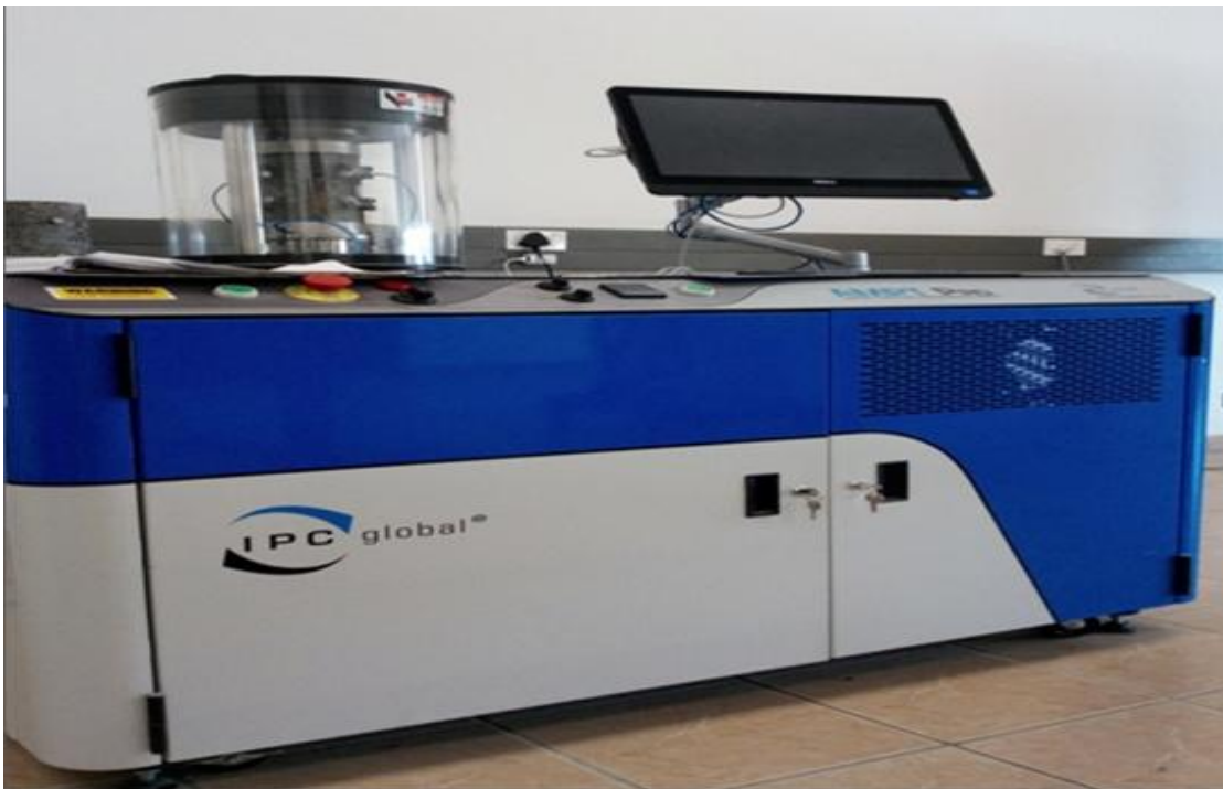
Figure 5.9. AMPT Machine Containing a Cylindrical Asphalt Specimen (Source: Author, 2019)
