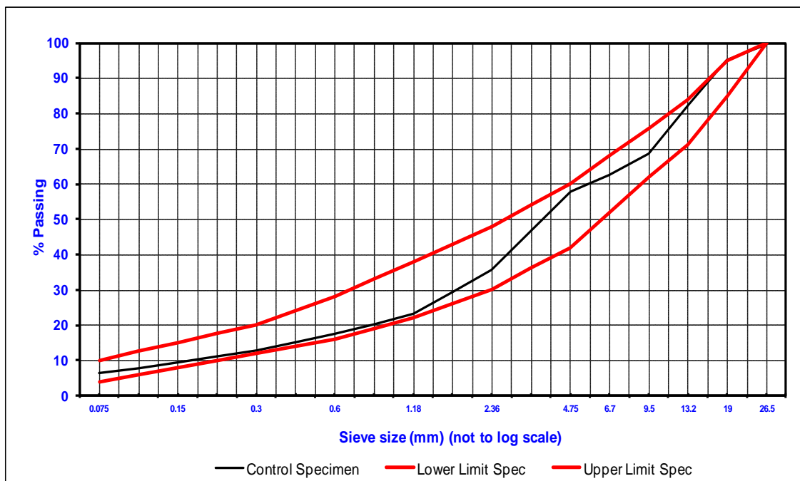
Figure 4. 3. Grading Envelope Graph of the Virgin Materials (Source: Author, 2019)
