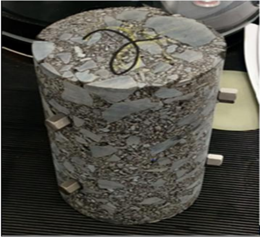
Figure 5.8. Asphalt Cylindrical Specimens (Source: Author, 2019)
