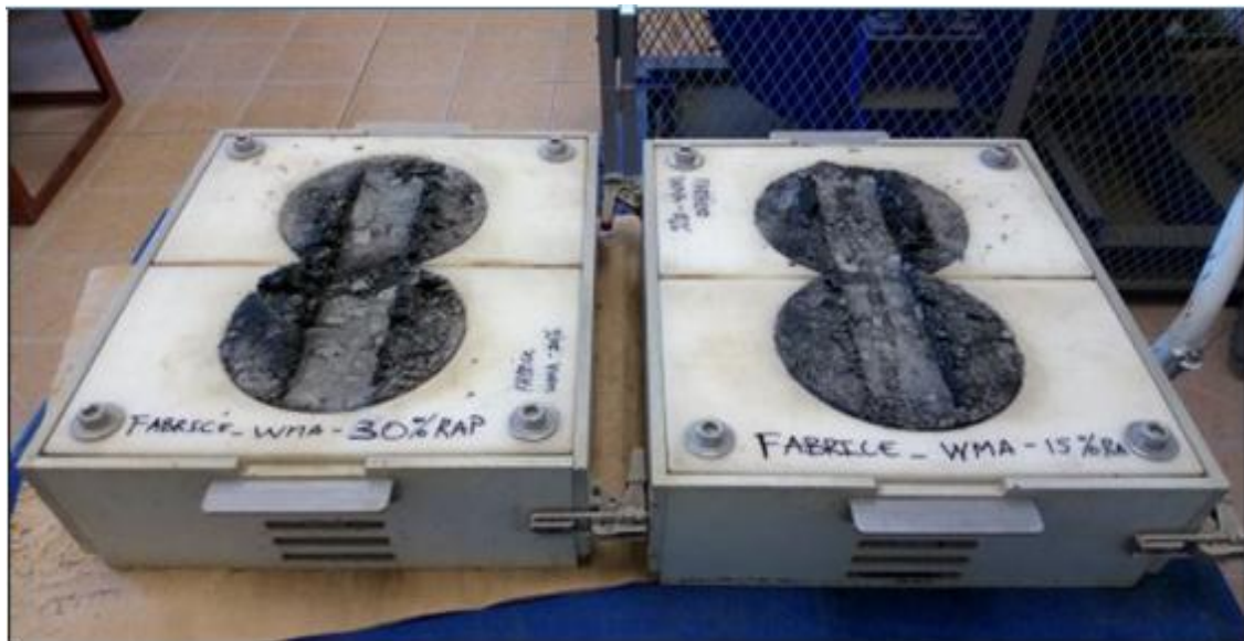
Figure 5.7. Asphalt Mixture Specimens Subjected to Hamburg Wheel-Tracking Test (Source: Author, 2019)
