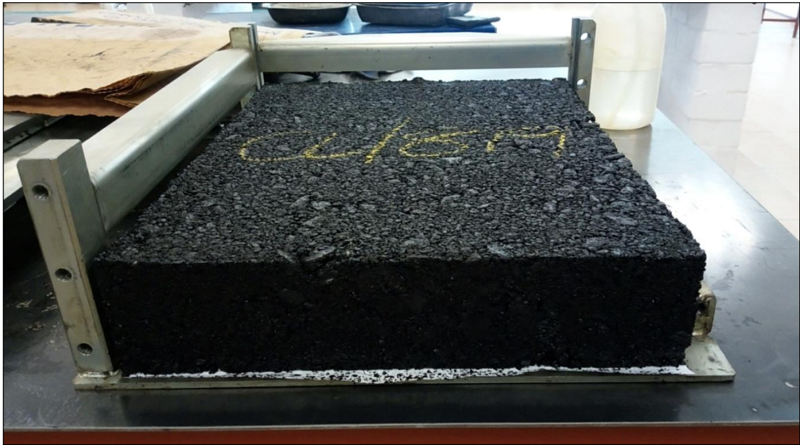
Figure 5.13. Compacted Asphalt Mix Slab (Source: Author, 2019)
