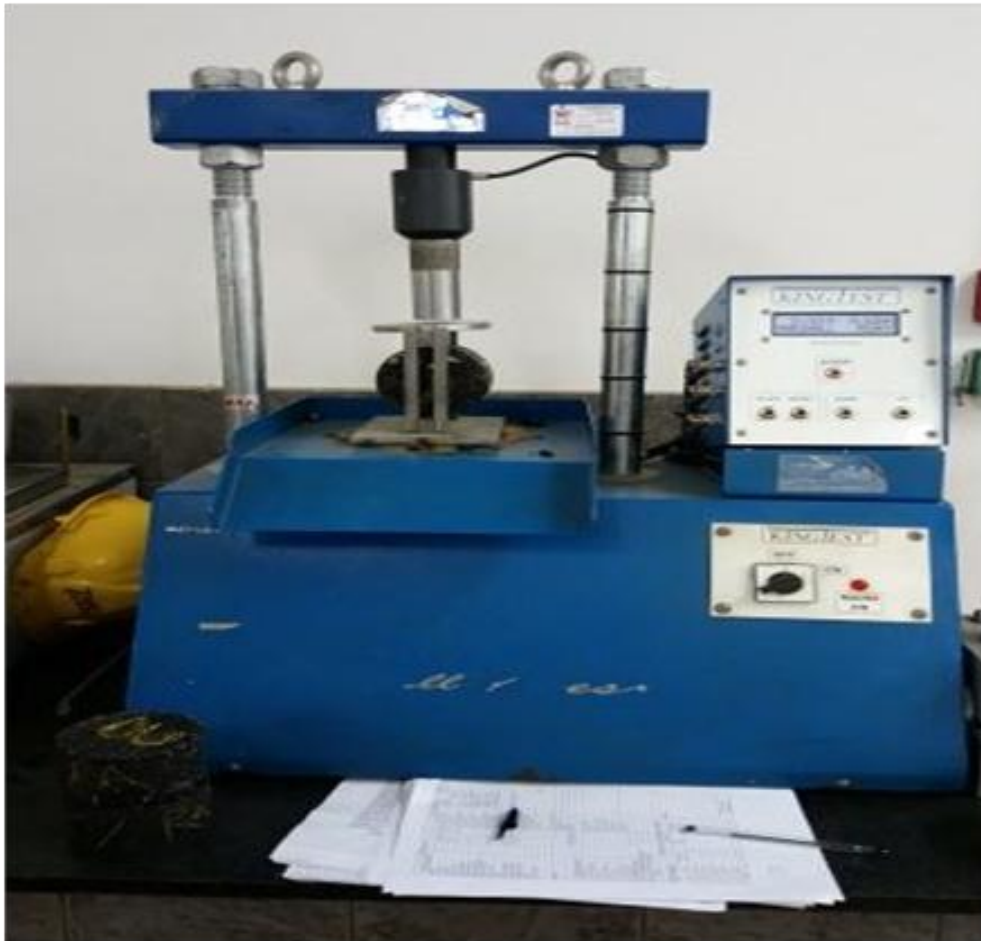
Figure 5.3. Asphalt Mix Specimen Configured in the ITS Test Machine
