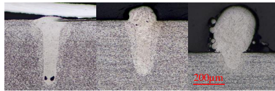
Figure 61: Cross-sections showing keyhole porosity and irregular surface of single tracks without powder (left), layer thickness of 120 \mu\text{m} (middle) and 300 \mu\text{m} (right) at 340 W laser power and 0.6 m/s scanning speed
