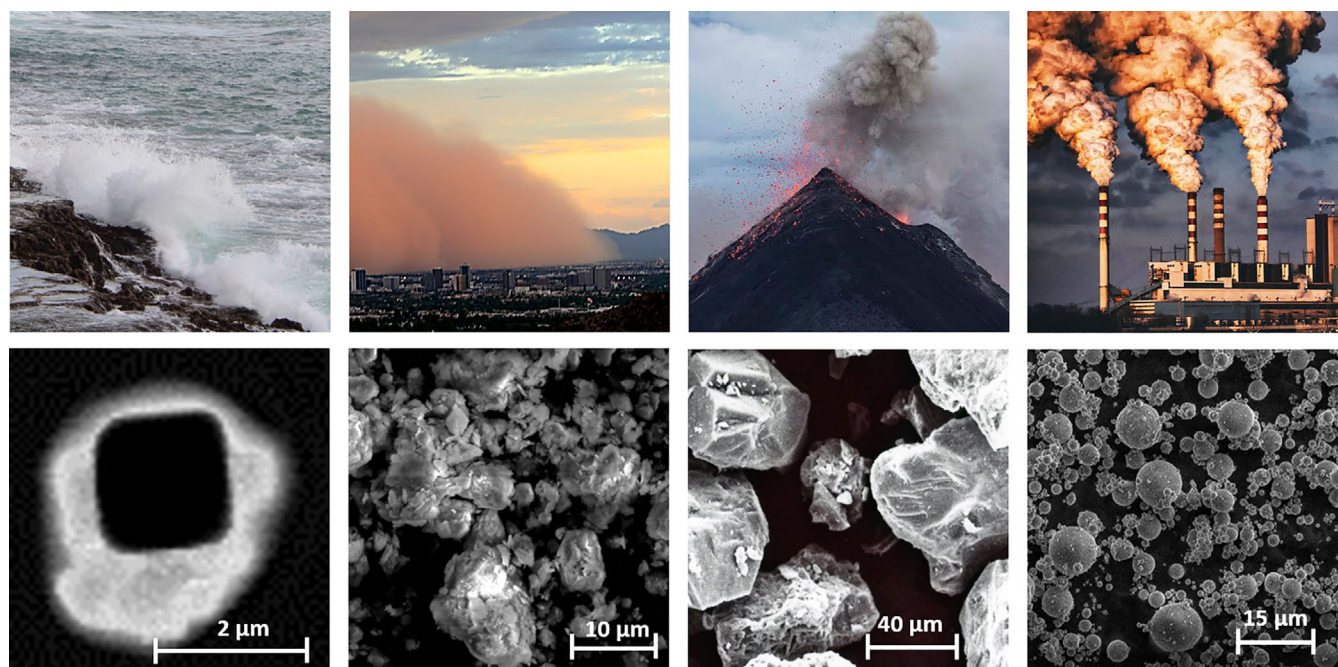
FIGURE 1 Top: Sea-spray aerosol, desert-sand dust, volcanic ash, and fly ash are sources of aerosols (photographs under Creative Commons). Bottom: Matching scanning electron microscope images (not at the same scale) showing the wide variety of aerosol sizes and shapes. Micrographs courtesy USCD/NSF-CAICE (Vicki H. Grassian) and Skidmore College/NSF-CAICE (Juan G. Navea)
