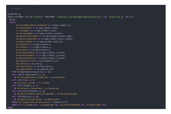
Figure 1. Stored Procedure: Server-side
