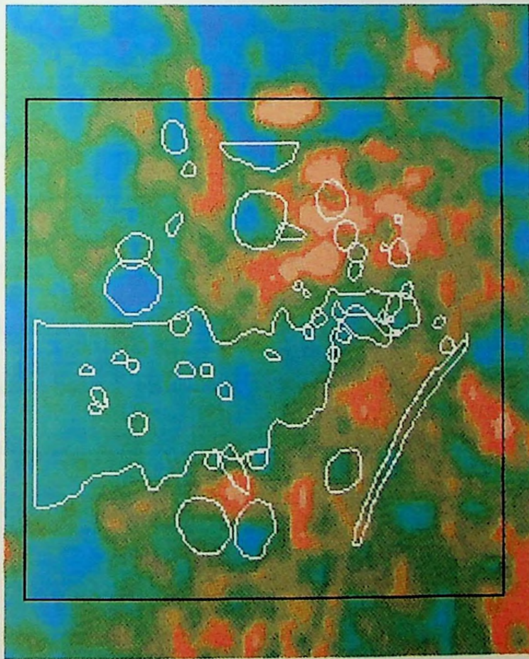
Pseudocolor CIR composite with unsupervised 80 classes Gaussian equalization enhancement 1997 imagery. Note the spatial correlation between the mapped Polytrichum sp. association and the image processed imagery. Y2 WVva.
