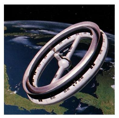
Figure 2.1. *von Braun's Space Station 1952*. This artist concept by Chelsey Bonestell depicted Dr. Wernher von Braun's early space station concept, a 250-foot-wide wheel that would rotate to provide artificial gravity. Von Braun was the first center director at NASA's Marshall Space Flight Center in Huntsville, Alabama. Image Credit: NASA/MSFC (Bonestell 1952).
