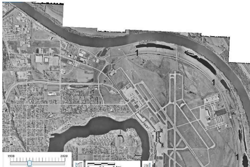
Figure 33: Roughly the same area as above, but in 1991. The airport has expanded significantly behind a new levee (marked with 1s). The river has been constrained to a ≈constant width channel by Army Corp structures. A close look shows small indentations that likely represent small scour pits down-flow of the wing dikes. Much of the point bar area of exposed sand bars is now on the protected side of the levee, but remnants are evident in the air photo. These sand bars would influence the shallow groundwater flow under the airport. Note the residential development in the area.
