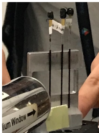
Figure C5. Set-up for XANES measurements of air-free solutions in quartz capillaries.
