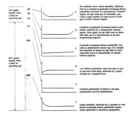
*Note.* The vertical axis represents the conditional probability of failure and, the horizontal axis represents operating age since manufacture, overhaul, or repair. The percentages show the percentage of items studied that fell into each of the basic patterns. Reprinted from *Reliability-Centered Maintenance* by Nowlan & Heap, 1978, Office of Assistant Secretary of Defense. In the public domain.
