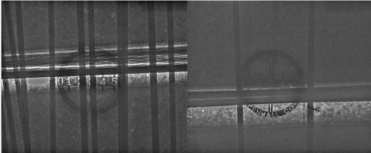
Figure 45: Internal Duct Specimen: Duct with strands 1ft away from end block (Left) and 5ft away from end block (Right)
