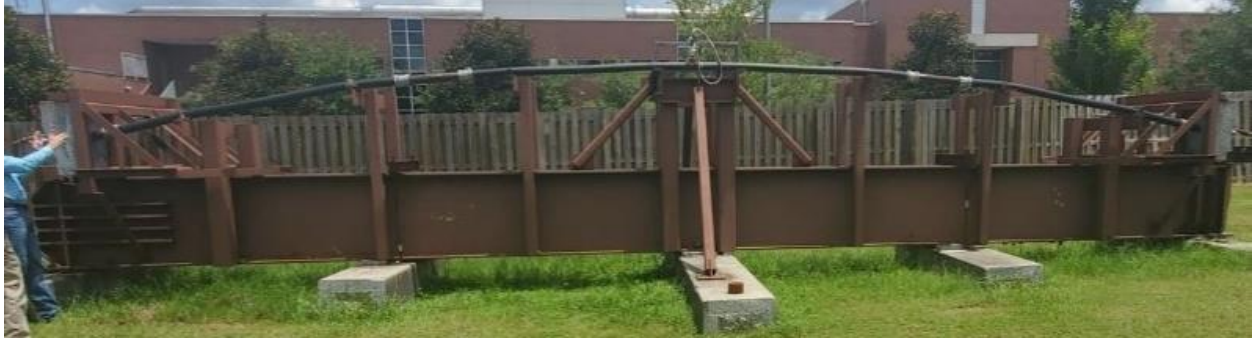
Figure 31: Filled External Tendon Mock-up
