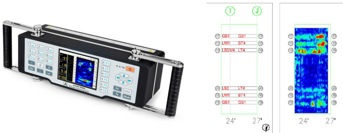
Figure 91: (Left) A1040 MIRA device, (Right) results from the deviator blocks (left is defect key and right is the UST scan) (Hurlebaus, Hueste, Karthik, and Terzioglu, 2016)
