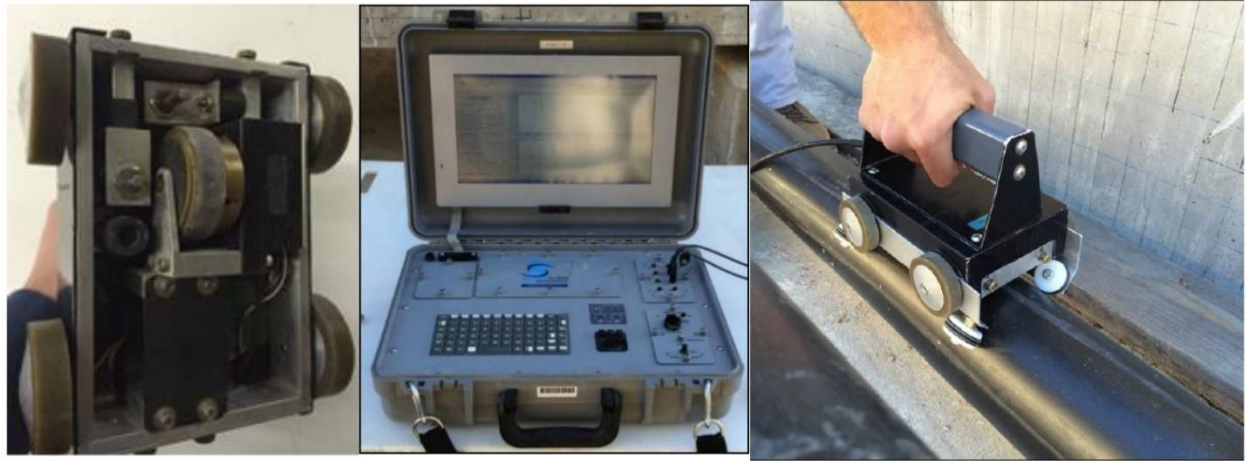
Figure 8: (Left) Shows the IE scanner test head, (Middle) Shows the PC data acquisition platform, (Right) Shows the IE device in use on an external duct (Hurlebaus, Hueste, Karthik, and Terzioglu, 2016)
