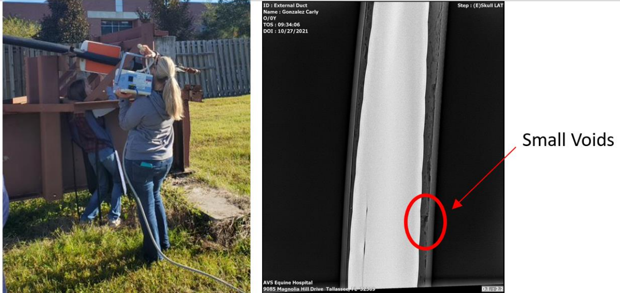
Figure 40: Specimen 2: Filled Duct Results
