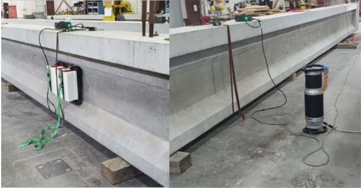
Figure 42: YXLON X-Ray Machine on Internal Duct Specimen
