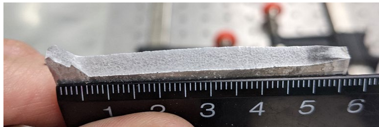
Fig. 26 Close-up image of the crack surface on specimen 3.
