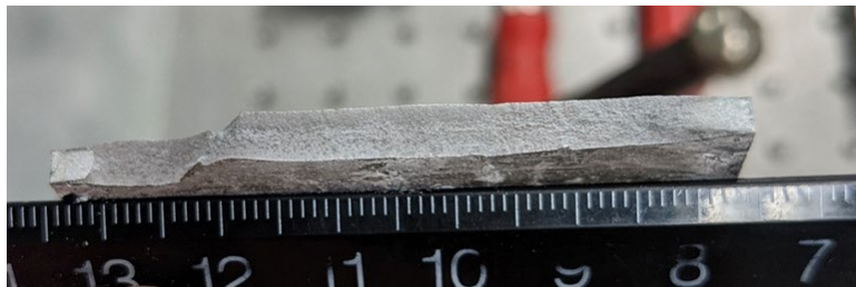
Fig. 23 Close-up image of the crack surface on specimen 2.
