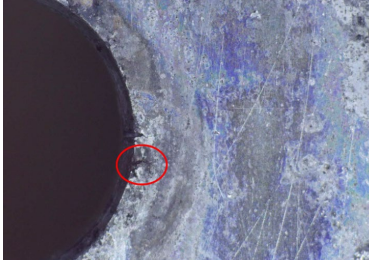
Fig. 24 Close-up image showing a secondary crack parallel to the main crack at 36,000 cycles.
