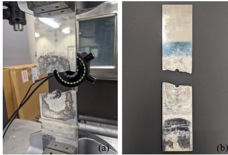
Fig. 18 (a) First specimen just after failure (b) First specimen removed from tensile machine.
