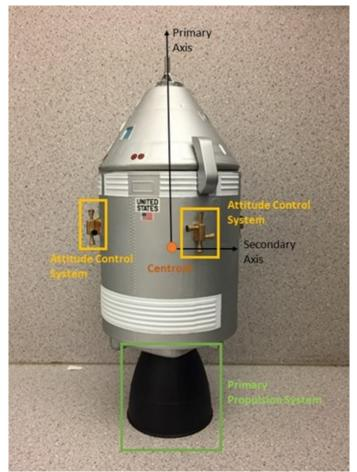
Figure 15. Detected and identified components of spacecraft model using CNN
