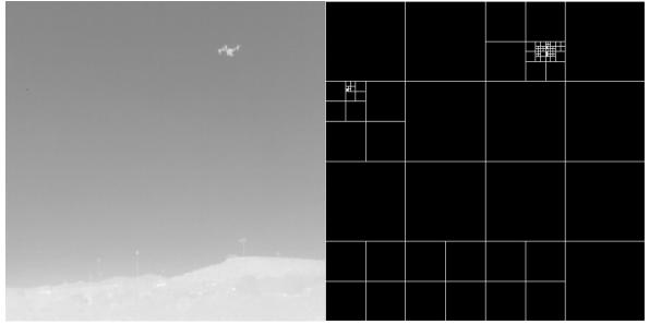
Figure 13. Quadtree deconvolution of IR image, identifying a UAS and zero pixel
