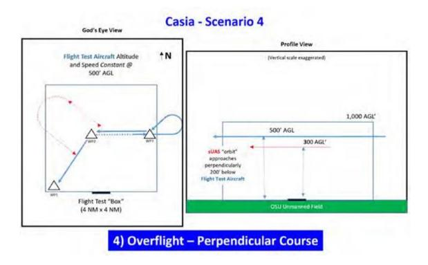
Test trials begin when the pilot of the SR20 GA aircraft announced over the radio when they were three minutes away from UAFS. To ensure proper testing parameters, the sUAS ownship established its autonomous waypoint missions before the GA entered the test box for each scenario.
