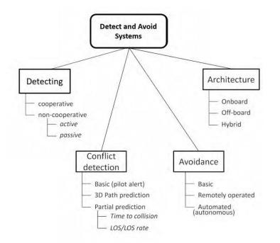
**Cooperative Technologies** – Cooperative sensor technology is used to receive signals of intent from other aircraft equipped with compatible avionics and to determine their position. Cooperative sensors usually have larger range than non-cooperative technology and are more reliable.
