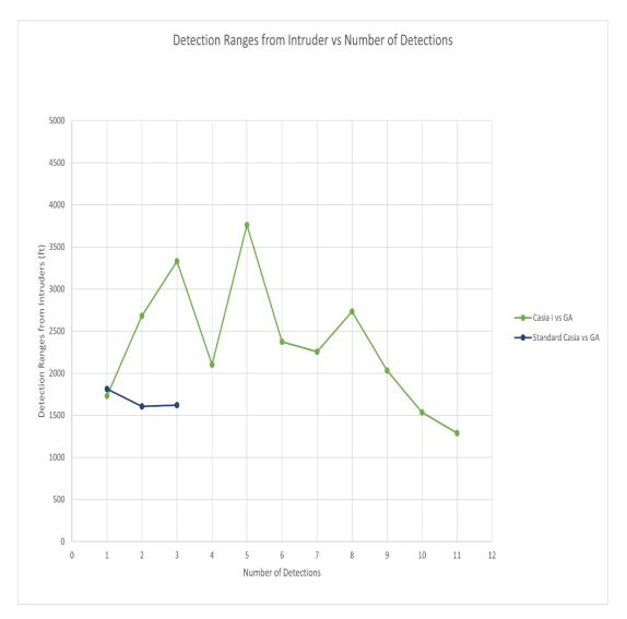
The standard CASIA provides a well-rounded system when it comes to initial DAA ranges, however, the 70 % larger lens size allows the CASIA I to outperform standard CASIA by number of triggered detections and range. Testing results were used to test the optimization of the DAA systems and determine detection ranges. Although most testing used CASIA I, given favorable weather, both systems performed well with detecting collision-course intruders within the
