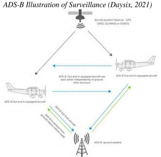
New advancements in commercial ADS-B have allowed it to be integrated into sUAS with minimal size/weight/power impacts. Use case examples for using transceivers for DAA can found elsewhere (Harvey & O'Young, 2015; Mitchel et al., 2020). Due to its limitations in tracking uncooperative aircraft, ADS-B is not an all-around solution, however. Additional onboard sensors should be paired to identify aircraft without ADS-B and other air-to-air conflicts, such as birds.
