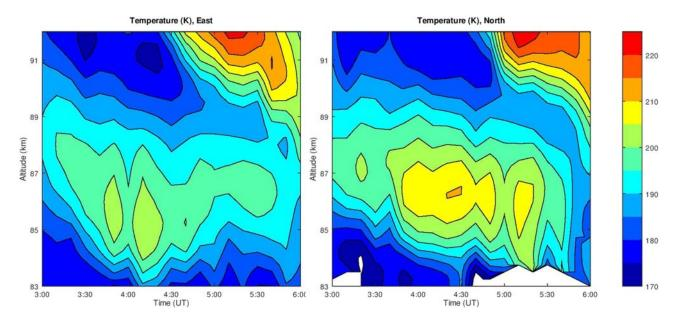
Figure 6. The USU Na lidar measured the time variations neutral temperature within the OH layer from east-pointing laser beam (left) and north-pointing laser beam (right) during the wave "blocking" event on the night of 11 September 2016.
