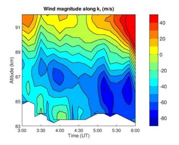
Figure 7. The USU Na lidar measured temporal variation of the horizontal wind projected onto the propagation direction of the "blocked" small-scale wave.
