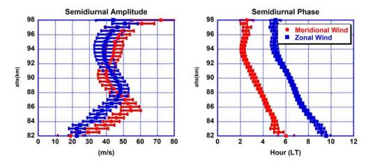
Figure 9. The Na lidar measured semidiurnal tidal amplitude and phase profiles of zonal and meridional wind during the 09-12 September period.
