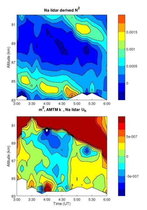
Figure 8. The calculated temporal variations of the Brunt-Väisälä frequency square (top) and the vertical wavenumber square (bottom) of the "blocked" small-scale wave, based on the AMTM and the Na lidar observations.
