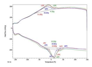
Fig. 7 DSC pattern of the NiTi stent after the heat treatment.
