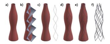
Fig. 2. (a) Base surface from mimicked patient data, b) reference surfaces for the mesh, c) baseline obtained from the intersection between the base surface and reference d) 3D wireframe with circular profile following the base surface, e) complete stent on the base surface, f) final stent.
