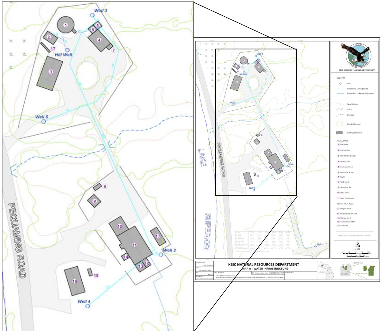
Figure 3. Site Plan of the KBIC hatchery. The map view of the Site Plan depicts the production wells, piping connecting the wells to the two head tanks (north and south head tanks), and structures currently present at the KBIC hatchery site. The full-size map image is provided in appendix B.
