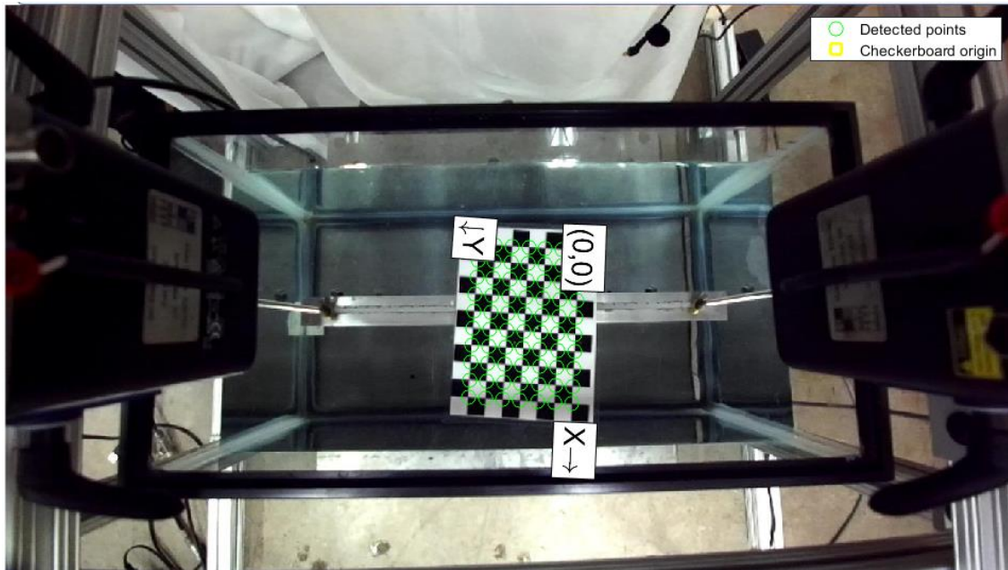
Figure 4.3: Checkerboard Calibration of Zed2 camera at water level to acquire camera intrinsic
