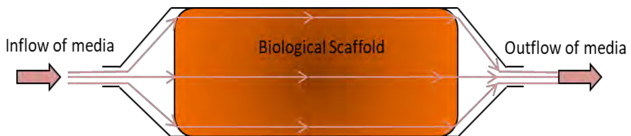
Figure 3.1: Diagrammatic representation of a forced perfusion based bioreactor.
