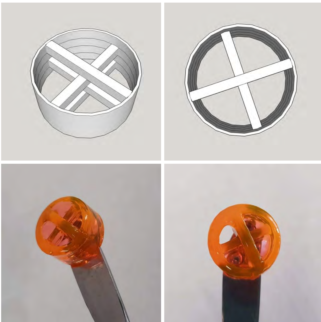
Figure 4.8: Images of a 20% PEGDA hydrogel scaffold, 3D printed using the developed visible light 3D bioprinting system at a 100 \mu\text{m} layer height with an intended outer diameter of 17.5 mm (Actual diameter 19 mm) and intended height of 12 mm (Actual height 12 mm).
