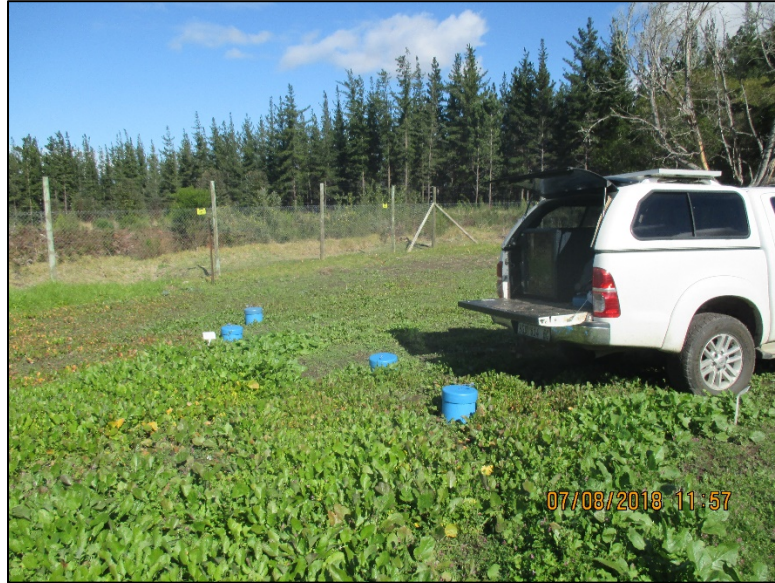
Figure 3.8: Two gas canisters placed in a conventional plot and two placed in an organic plot during sampling.
