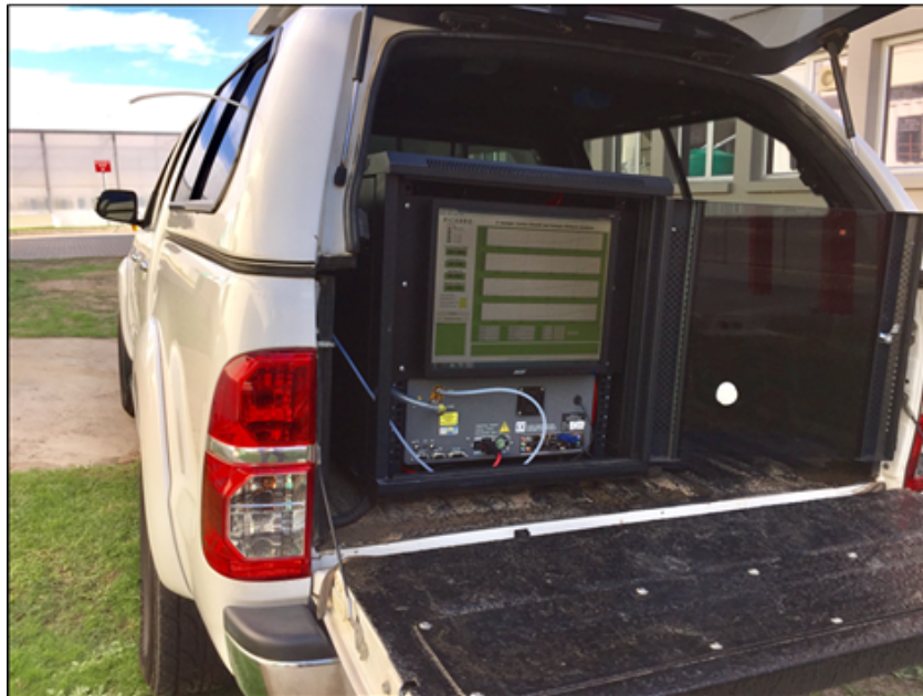
Figure 1.3: Picarro G2201-i gas analyser, presently the only such instrument in South Africa. The instrument is capable of identifying and quantifying CO 2 and CH 4 isotopes.
