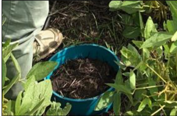
Figure 3.10: The base part of the canister that's hammered into the soil two days prior to sampling. The base is specially fitted to the chamber which is attached to the lid, and are airtight while attached.
