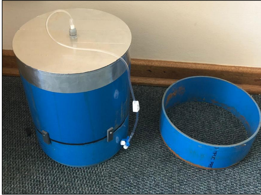
Figure 3.6: Static chamber used to trap emitted gas from the soil in Bethlehem. The canisters are different from the one used in study area one and they belong to the University of Free State (UFS).
