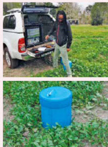
FIGURE B24.2. Top: Picarro in truck used to analyse CO 2 and CH 4 concentrations in gas canisters in the test crop-plots. Bottom: Special designed gas canister used to accumulate GHG in the headspace
