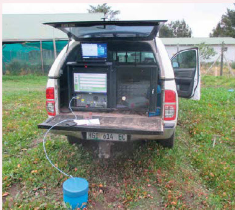
FIGURE B24.2. Top: Picarro in truck used to analyse CO 2 and CH 4 concentrations in gas canisters in the test crop-plots. Bottom: Special designed gas canister used to accumulate GHG in the headspace
