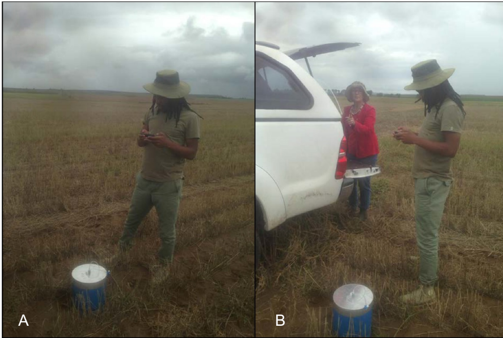
Figure 3.11: Canister closed during fifteen minutes gas sampling. A stop watch is used to ensure exactly fifteen minutes in each plot. During the fifteen minutes, atmospheric temperature and soil temperature were collected too.
