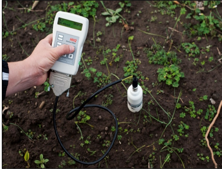
Figure 3.7: Theta probe placed next to canister before sampling to measure soil moisture content in percentage, 0% being very dry and 100% being very moist; this is too establishes the correlation between soil moisture and emissions. It measures only the top 6cm of the soil.
