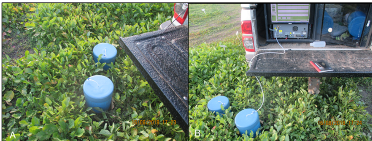
Figure 3.9: (A) Two gas canisters in a field during sampling. (B) Two gas canisters in the field during gas analyses, the Picarro is suctioning the gas trapped in the canister during emissions.
