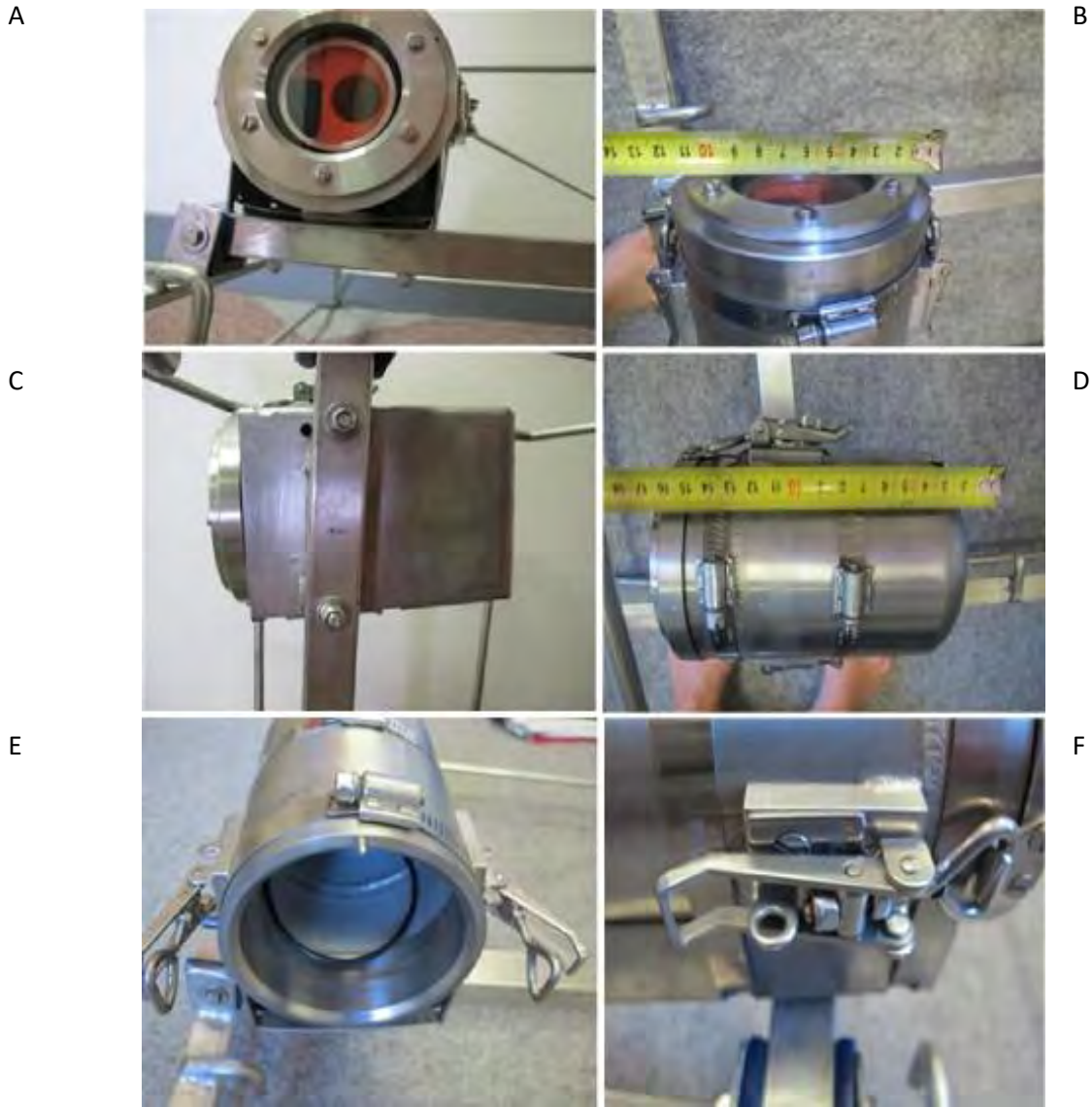
Figure S5.8: Camera housing A) front view, B) top view, C) from the base with a view of the cradle, D) attachment clamps, E) inner cavity and F) clamps that secures the detachable front form the rest of the housing.
