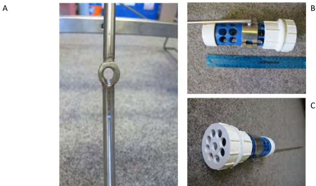
Figure S5.9: A) Bait arm seat, B) arm and C) bait canister
