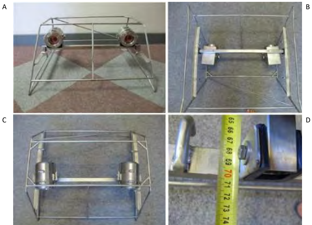
Figure S5.7: sBruv frames side view, B) view from bottom, C) view from the top and D) camera base with polymer lined cradle.
