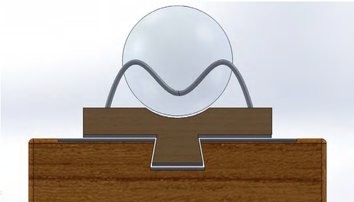
Finally, a front elevation with exaggerated clearances; note the cladding is recessed, here, but this is not necessary in practice if the dovetail is routed to a greater depth.
