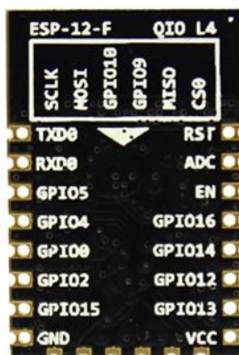
Figure 4-5 ESP-12F pin description
